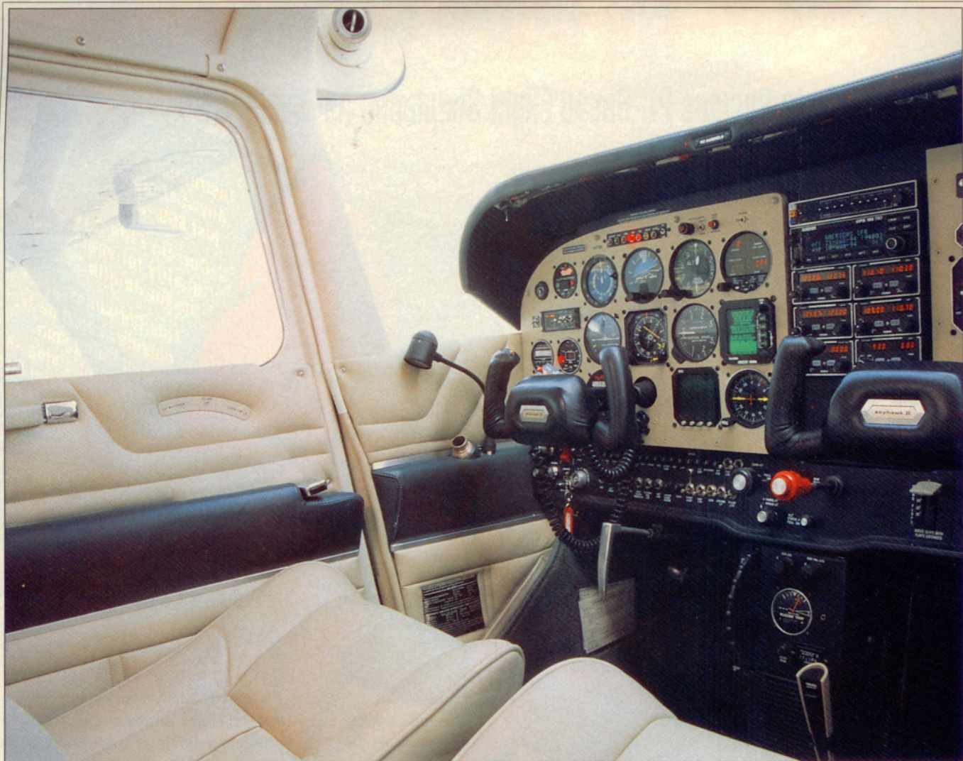
An aluminum rail (below) forms a sturdy arm rest and ledge that runs the length of the cockpit (above) and houses the door latch, additional air vent, and lamp. Handy pockets between the seats carry charts (right).
