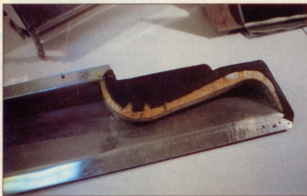
An aluminum rail (below) forms a sturdy arm rest and ledge that runs the length of the cockpit (above) and houses the door latch, additional air vent, and lamp. Handy pockets between the seats carry charts (right).
